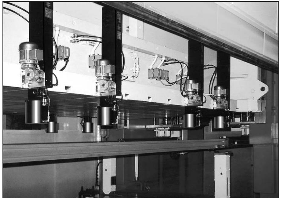
Rapid clamping system with pusher chain fastened to the press ram of a double column press. A hollow piston cylinder serves as clamping element.
