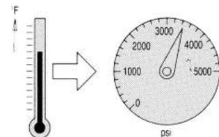
Another strange effect is pressure change due to temperature change of a closed system. In fact, pressure changes about 80 psi per 1° F! Be careful of excessive temperature changes, especially increases. Use a Pressure-Relief Valve for safety.
