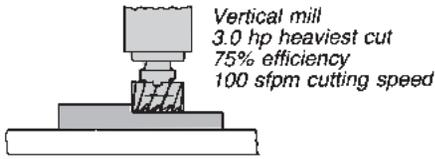
$$\begin{aligned} \text{Cutting force} &= \frac{3.0 \text{ hp} \times .75 \times 33,000}{100 \text{ sfpm}} \\ &= 743 \text{ lbs} \end{aligned}$$
