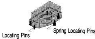
Evaluate workpiece-loading procedure and clamping sequence. Loading and clamping can be completely automatic, or involve some manual steps. To position the workpiece against locators, spring-loaded positioners (above) are often helpful. Sequence Valves are extremely useful to position hydraulically with push clamps before clamping. Total positioning force should be 30-50% of the workpiece's weight to overcome friction.
