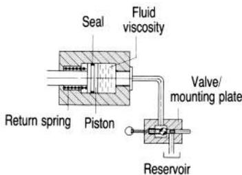
2. Large fixtures with long tubing runs or flow restrictions. Return speed is adversely affected by: (1) pressure drop in tubing and hoses; (2) pressure drop in valves; (3) high fluid viscosity, especially at lower temperatures; (4) frictional force at piston seals, especially when clamped for an extended time, which displaces the fluid film on cylinder walls.
