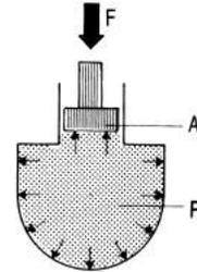
via hose, tubing, or drilled passages. When hydraulic pressure acts on a clamp's piston area, it generates external force according to the physical relationship  $F=P \times A$ :
