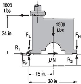
The equations below solve for unknown forces assuming that for a static condition:
