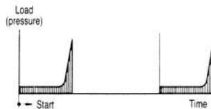
Extending time is fairly easy to calculate, knowing fluid required by each clamp and the power units flow rate, using the formula below. One obvious way to reduce clamping time is to set clamps as close to the workpiece as possible, to use as little stroke as possible.
