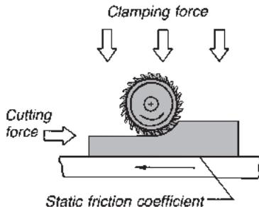
$$\text{Clamping force (lbs)} = \frac{\text{Cutting force (lbs)}}{\text{Static friction coefficient}} \times \text{Safety factor (usually 2)}$$
