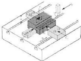
Use positive stops to resist machining forces, rather than relying just on clamp forces. With well-placed locators, you can use smaller clamps.
