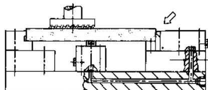
Our Roemheld line pioneered the ever-increasing use of manifold mounting: supplying fluid to clamps through passages drilled in the fixture, rather than through tubing or hoses. Manifold mounting, which requires specially designed clamps, allows designing totally "clean" fixtures without chip traps. Also, manifold mounting lets you put clamps closer together and in tighter spots, often letting you put more workpieces on a fixture.
