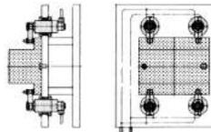
2. Tubing lines underneath fixture plate. Running tubing lines below the working area is an improvement on option 1. Advantages: no chip traps in working area; more freedom to position clamps with tubing out of the way. Disadvantages: a large base-plate area is still required; more complicated fixture construction.
