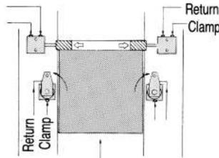
3. Machine-tool interlock. In automated systems where timing and synchronization are important, double-acting clamps are the best choice. By installing pressure switches in both clamping and return lines, a machine controller knows exact clamp status at all times.
