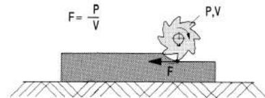
$$Cutting\ force\ (lbs) = \frac{Heaviest-cut\ horsepower \times Machine\ efficiency\ \% \times 33,000}{Cutting\ speed\ (sfpm)}$$
