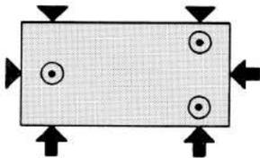
Choose clamping points that are backed up by solid stops or rests to resist clamping forces. Clamping forces can distort a workpiece unless counteracted by firm supports.
