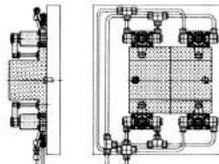
1. Tubing lines on top of fixture plate. This is the oldest, most traditional method of supplying fluid to hydraulic clamps. Before manifold mounting, using tubing was about the only option available. Advantages; less baseplate machining is required; more freedom to position clamps with tubing out of the way. Disadvantages: chips are easily trapped in tubing lines; a large base-plate area is required; exposed tubing is subject to damage.
