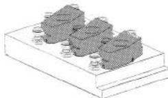
Decide how many parts you want to place on the fixture. For example, to place three workpieces on the above fixture, super-miniature Swing Clamps are necessary. With only one workpiece, just about any clamp would do.
