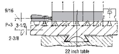
Excess force can cause fixture and machine-table distortion or even damage. Even a small hydraulic clamp can generate tremendous stresses (S). In the example above, three
