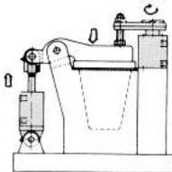
1. Moving linkages or retracting heavy loads. For a quick, positive return when weight is too heavy for spring return.
