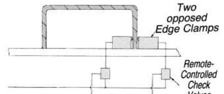
In the example above, the two opposed clamps allow the workpiece to float between them. Pushing on one clamp encounters no resistance because fluid just shifts to the opposing clamp (if the check valves were not present). Do not let equal-force clamps oppose each other without Remote-Controlled Check Valves.
